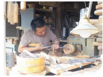
Shaping the wood using an electric wheel and a wood plane
